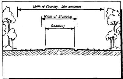
3 **Typical Road Cross Section**: Roadway and daylighting can almost always be accommodated within a maximum cleared edge to cleared edge width of 40 m. Excessive road clearance does not enhance drying from the sun.
