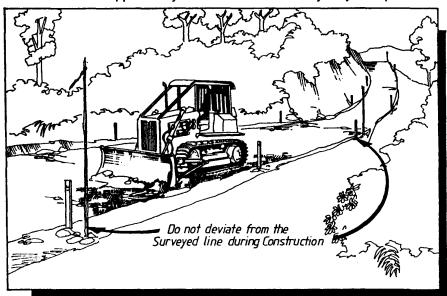
2 Key Standard No. 9: Maximum cleared forest road width is 40 metres. The maximum cleared forest edge to cleared forest edge width on main roads is 40m. Trees cleared for roading should be felled directionally along the road corridor. to avoid canopy damage to the standing forest at the edge of the corridor. Minimise the amount of vegetation cleared during road construction to assist wildlife passage and minimise canopy clearance.
